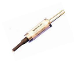
The Fiber Coupled Si Photodiode is based on a unique configuration that features high sensitivity, low noise, and high optical coupling efficiency. The component integrates a fiber with a silicon PIN photodiode for signal detection with little optical loss. The response is analog. Our design minimizes component assembly costs and module footprint while increasing stability over a wide temperature and wavelength ranges.
